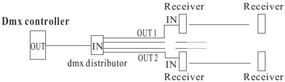
**Receiver can not more than 32 units on one out channel
