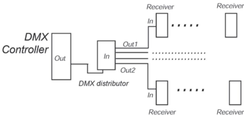
You can run a maximum of 32 units (receiver) per output channel.
